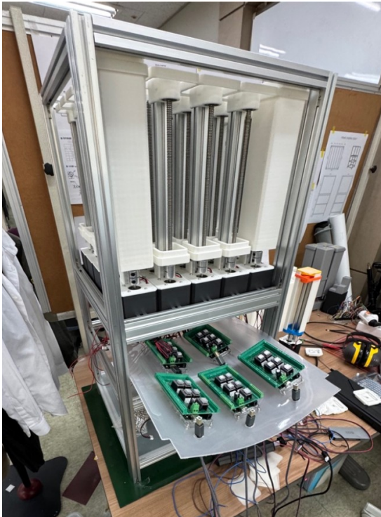
Figure 4-3. Partially assembled 5×5 actuator frame during installation of five Arduino Mega boards.
