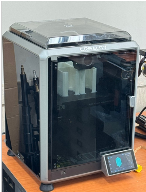
Figure 4-1. An FDM printer (Creality K1C) used for fabrication of prototype components.
